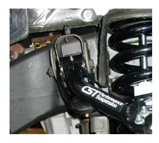
15. GREASE URETHANE BUSHINGS AND INSTALL INTO UCA PIVOTS THEN GREASE STEEL CRUSH SLEEVES AND INSTALL INTO URETHANE BUSHINGS. INSTALL GREASE FITTINGS INTO UCA PIVOTS. INSTALL BALL JOINTS INTO UCA WITH 5/16" x 1 1/2" BOLTS AND HARDWARE, THE BALL JOINT AND THE SPACER SLIPS INTO THE CENTER OF THE TWO PLATES ON THE END OF THE ARM. THE SPACER GOES ON TOP OF THE BALL JOINT.
