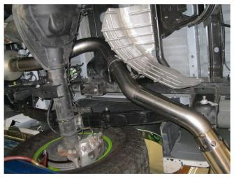
**Step 6.** Next Install the Tail Pipe Assembly in a similar fashion using the supplied 5.00" clamps and by fitting the welded hangers into the rubber insulators.
