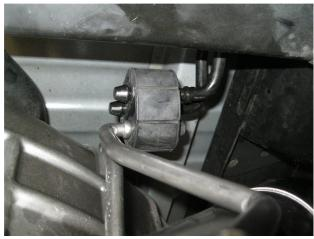
**Step 2.** Begin installation of the Magnaflow system by clamping the Inlet Pipe to the outlet of the DPF using a supplied 4.00" clamp and fitting the hangers in the rubber insulators (leave all clamps loose for final adjustment of the complete system).
