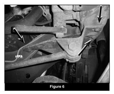
18. Install the new provided pitman arm (083401R or 083403R) on the steering sector shaft. Use the marks made on the factory arm as a guide. Fasten the pitman arm with the original sector shaft nut/washer. Torque nut to 185-200 ft-lbs.
