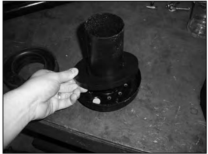
15. Reassemble the strut. Make sure to line up all of the alignment marks. Fasten the strut rod with the original nut. Torque nut to 35 ft-lbs.
