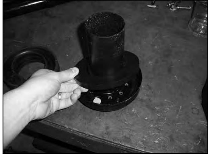
15. Rotate the top plate 180 degrees. This will allow the lower bar pin to reassemble in the lower control arm smoothly. Note the before and after strut pictures.
