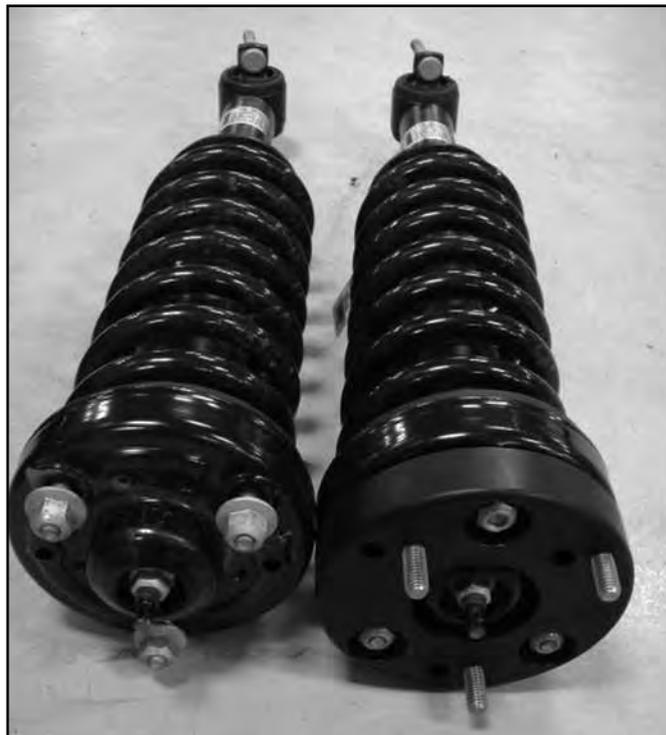
18. Install the modified strut assembly into the upper frame mount by aligning the studs in the new spacer with the original mounting holes. Loosely fasten the strut with the provided 7/16" nuts and washers. Note: The driver's side will have the correct notation on the spacer, the passengers side notation will be incorrect due to model year changeover in 2014.
