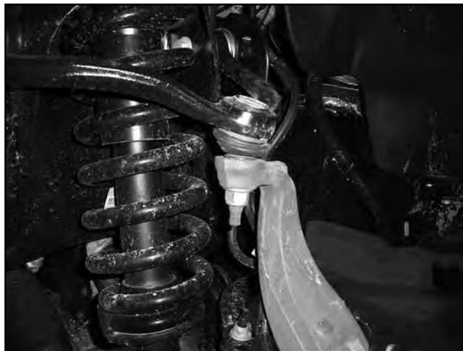
10. Support the lower control arm with an appropriate jack. Remove the three upper strut mounting nuts at the frame. (Fig 6) DO NOT remove the center strut rod nut. Save nuts.
