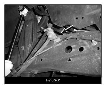
9. Disconnect the front sway bar links from the sway bar and frame (Fig 3A,B). Remove the links from the vehicle and discard. Save hardware. Note: Some early model vehicles had sway bar link mounts below the frame. The newer style frame mount is shown in Fig 3A
