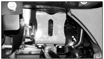
36. Install the sway bar link ends in the original axle mounts and secure with the OE hardware.
