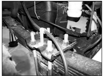
69. Reattach parking brake cable bracket to the spring plate. If more slack is needed remove the cable from the rear-most cable ring on the frame rail (Fig 16).
