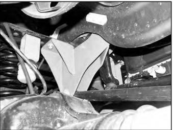
22. Pull the OE front bump stops free from the bump stop cups and remove the bolt mounting the cup to the frame (Fig 8).
