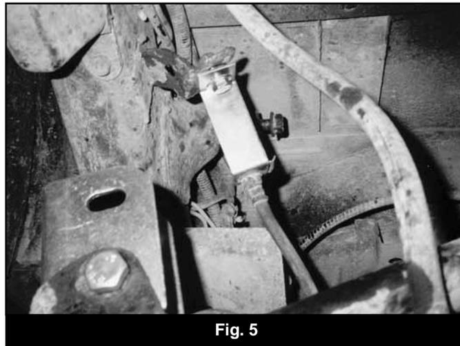
25. Support differential; remove spring mounting bolts, u-bolts and remove springs.
