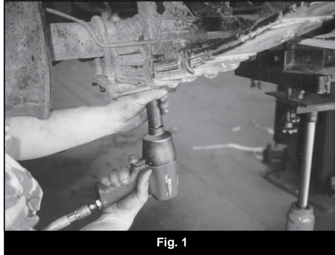
7. Position u-bolt plates and install the new u-bolts, washers, nuts and new bump stop contacts. These are retained to the axle by the outer most u-bolts on each side.
