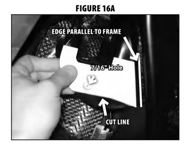
37. Drill a 7/16" hole at the marks made on the factory UCA mounts. Trim along the cut line, making the bottom-rear edge straight (Fig 16B).
