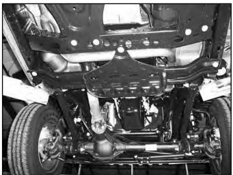
23. Remove the outer transmission crossmember mounting bolt on each end of the crossmember (Fig 10). Retain the mounting hardware.
