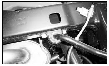
46. Install sway bar drop brackets with OE sway bar mounting bolts to frame rails. Brackets will be offset toward the rear (Fig 25R). Mark the hole to the rear of the existing OE holes.
