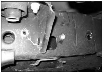
26. Use the provided fish wire to pull the 1/2" bolt tab (01797) through the frame (Fig 16R). Note: Do not put a washer on the bolt tab.
