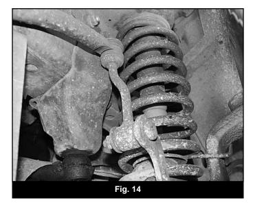
35. Disconnect the steering stabilizer from the axle and retain hardware. If replacing, remove the steering stabilizer from the drag link by removing the nut and dislodging the tapered stud with a pickle fork (Fig 15).
