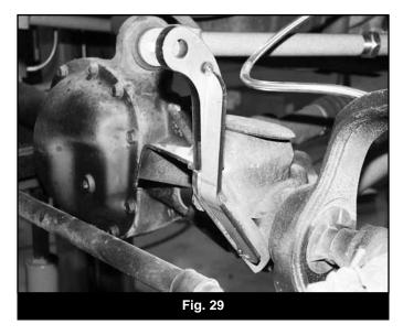
72. With the link mount parts correctly in place finish weld the components to the axle. Weld all around the point where the original mount meets the new mounts as well as the full length of the gusset where it meets the new and original link mounts (Fig 30). Note: Weld the back side of the gusset for best weld penetration and aesthetics.
