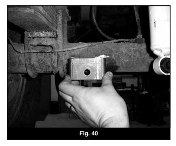
29. Position the new shock mounts so the flat shock mount surface is parallel to the centerline of the shock (Fig 41). This will ensure that the shock bushing will run square in the shock eye at ride height. Tack the brackets into position.
