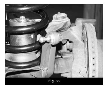
82. Install the provided upper u-bracket (01325) to the sway bar using the original link mounting hole with a 7/16" x 1-1/2" bolt, nut, 7/16" SAE and 7/16" USS washers (BP 718). Install the bolt up through the u-bracket with an SAE washer into the sway bar. Fasten with the nut and USS washer. Position the bracket so that the thru-holes are parallel with the stud on the axle (Fig 34). Torque to 50 ft-lbs.
