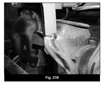
70. Repeat the link setup procedure on the passenger's side of the vehicle (Fig 28). With both pieces tacked in place check the relationship between the two mounts to see that they are the same. Measure the inside distance between the tops of the links and the bottoms of the links to see that they are the same (approximately 38-1/2").
