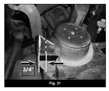
74. Position the new provided stabilizer mount (01354) on the top of the original mount so that the hole is to the driver's side and the front surface is aligned to the line marked on the top of the OE bracket (Fig 32). The will butt up to the passenger's side link mount that was just installed.
