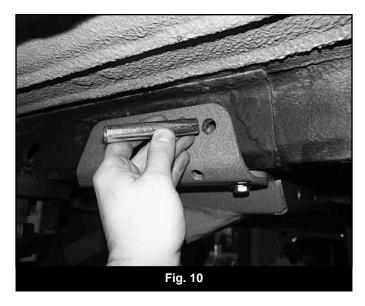
25. Install a 3/8" USS washer on a 7/16" x 4-1/2" bolt (BP 715) and insert it into the frame crush sleeve. Push the bolt and sleeve all the way into the frame so that the sleeve is against the inside surface of the frame and the bolt is sticking out of the inside 7/16" hole. Fasten the bolt on the inside of the frame with a 3/8" USS washer and 7/16" nut from bolt pack 715 (Fig 11). Leave hardware loose. Ensure that the bolt does not hit the fuel or brake lines. Reform these lines as necessary.
