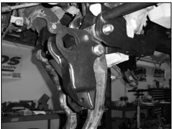
57. Remove the hub bearing and brake dust shield from the factory steering knuckles (Fig 34). Be sure to note which hub goes on which side of the vehicle. Locate the hub o-ring inside the knuckle hub bore. Using a small flat head screw driver remove the o-ring for use in the new knuckle (Fig 35). Save mounting bolts, o-ring, dust shield and hub, discard the knuckle.
