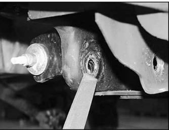
40. Locate the new front crossmember (02190). Install the crossmember in the front lower control arm pockets so that the two longer differential mounting tabs are on the driver's side pointing rearward (Fig 22). Fasten the crossmember with the original lower control arm hardware. Run the bolts from front to rear. Leave hardware loose.
