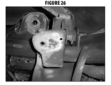
46. Locate the new provided bump stop brackets (02199). Place a bump stop bracket up to the original mount and line up the center of the two slots with the two holes in the factory mount. Using the third slot in the bracket as a guide, mark the center position to be drilled (Fig 27). Remove the bracket and drill a 7/16" hole at the mark.
