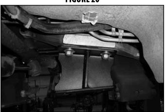
39. Inspect the inside factory control arm mounting holes. There will be a sharp lip left from the original control arm/hardware. Use a file or rotary grinder to remove the sharp lip left from the control arms (Fig 21). This will allow the new cross members to be installed easily.
