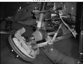
the CV axle from the hub (Fig 10). Mark the CV axle to indicate DRV side and PASS side.
