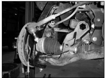
64. Position the provided CV spacer (02328 - Standard, 02329 - Narrow Track) between the CV shaft and the differential mounting flange (Fig 39). Fasten the CV and spacer to the differential flange with 10mm x 70mm socket head cap screws for standard track systems. Use 10mm x 50mm bolts and 10mm washers for narrow track systems. (BP 568 - Standard, 578 - Narrow Track). Use Loctite on the bolt threads and torque to 45 ft-lbs using a crossing pattern.
