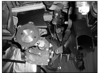
42. Install the new provided bump stops (M02096RB) on the new rear crossmember (02191) with 3/8" hex nuts, flat and lock washers (BP 539). Tighten hardware securely (Fig 24).
