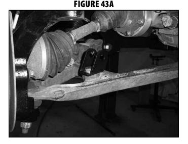
74. Locate the new front sway bar links (911109), small hourglass bushings (SB35BK) and 0.750" OD x 1.575" long sleeves (54587). Install the bushings and sleeves into the eyes of the links. Install the links into the new brackets on the lower control arms with 9/16" x 2-3/4" bolts, nuts and washers (BP 569). Run the bolts from front to rear and leave hardware loose (Fig 43b).
