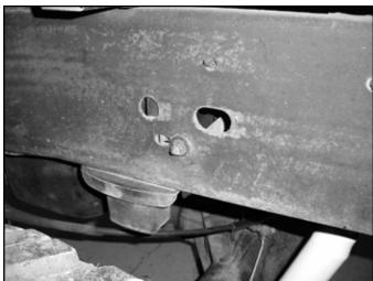
Support the center of the axle with a hydraulic jack. Remove the factory shocks from the axle and frame. Save hardware and discard
