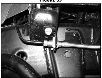
66. There are two threaded holes near the top of the steering knuckle neck on the back side. Using a provided wire clamp, 1/4" x 3/4" bolt and 1/4" lock washer (BP 590) loosely fasten the brake line to the lower threaded hole on the steering knuckle. Using the same fastener combination, attach the ABS line to the upper threaded hole. The hardware will be tightened once the line slack is set. (Fig 36A).
