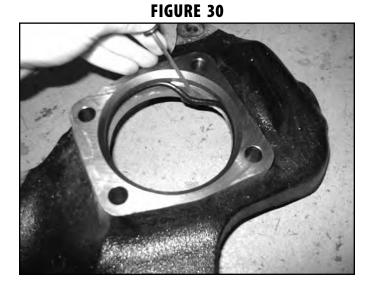
53. Locate the factory driver's and passenger's brake dust shields. They need to be modified to provided adequate brake caliper clearance. Make a cut line by following the straight edge on the caliper side of the shield all the way to the bottom edge of the shield. (Fig 31) Cut the shield along the line.
