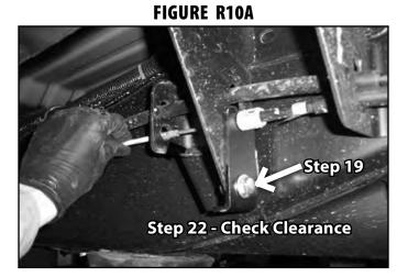
22. All model year trucks: Clearance the hole from the original e-brake location to clear the e-brake extension tube (if necessary). Insert the e-brake cable through the extension tube. (Fig R10b)
