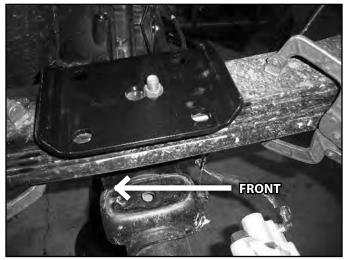
13. 3" & 5" Overload options: The Models equipped with overload leafs will need the separation block modified. Trim the anti-rotation tabs from the front side of block on both the inside and outside of the block. Use extreme care near the fuel tank, do not use any method that will create sparks if the block is not removed when modified. A sawzall is highly recommended. (Fig R6)
