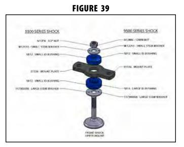
72. Install the front shocks in the vehicle. Fasten the lower mount with the provided 14mm x 70mm bolt, nut and washers (BP587). Fasten the upper bar pin bracket with 1/2" x 1-1/4" bolts, nuts and 1/2" SAE washers. Torque the upper bolts to 60 ft-lbs. Torque the new lower shock
