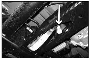
5. Unload the torsion bars but do not remove. Remove and save adjuster bolt/retainer block.
