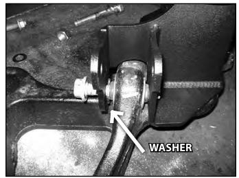
With both new torsion bar bracket installed on the factory control arms, install the control arms in the crossmembers. Fasten the control 45. arms with the provided 18mm x 120mm (front) and 18mm x 140mm bolts, nuts and 3/4" SAE flat washers (BP 585). Run the front bolts front-to-rear and the rear bolts rear-to-front. (Fig 27) Leave hardware loose. These bolts will be torque with the weight of the vehicle on the suspension.
