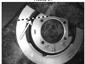
54. Install the hub assembly and dust shield into the appropriate steering knuckle. The ABS line will run out the top of the hub and behind the dust shield. (Fig 32) Fasten the hub to the knuckle with the factory bolts. Apply Loctite to the threads and torque the bolts to 125 ft-lbs.
