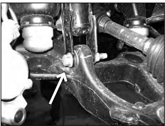
23. Remove the front and rear lower control arm bolts and remove the control arms from the vehicle (Fig 14) Save the control arms and mounting hardware.
