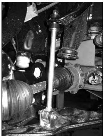
71. Locate the new provided BDS front shocks. Follow the diagrams for assembling the upper shock ends. (Fig 39) A small amount of grease will aid assembly.
