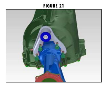
35. Locate the new passenger's side differential bracket (02371). Bracket has a single center gusset. Install the bracket on the existing studs on the passenger's side factory bracket. Fasten with the original nuts and washers. When installed the open side of the bracket will face inward and the bracket will taper down as it goes to the rear (Fig 22). Torque nuts to 65 ft-lbs.
