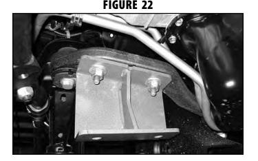
Locate the new driver's side differential bracket (02369). Bracket has two center gussets. Install the bracket to the 2 front original 36. differential mounting holes with the provided 12mm-1.75 x 40mm bolts and 1/2" SAE washers (BP 586), applying Loctite to the threads before installation. When installed the open side of the bracket will face inward and the bracket will taper down as it goes to the rear (Fig 23). Torque bolts to 65 ft-lbs.
