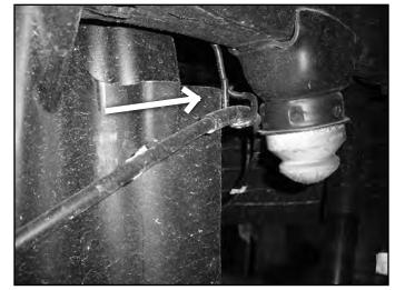
8. Push the ABS wire clips from the metal tabs just inside of the leaf springs. Remove the plastic clips from the ABS wire.(Fig R4)
