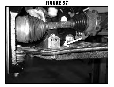
70. Install the new sway bar links into the new brackets and fasten with the provided 3/8" x 2-1/2" bolts, nuts and 3/8" SAE washers (BP 582). Leave bolts loose. Install a provided 7/16" washer followed by a stem bushing. Install the link end into the sway bar end and fasten with a second stem bushing, 7/16" washer and 7/16" nylock nut (BP 582). Tighten the 7/16" nut just until the stem bushings begin to swell. (Fig 38) Torque the 3/8" hardware to 30 ft-lbs.
