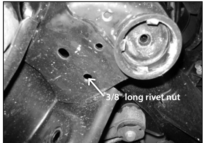
FIGURE 26B (REAR BUMP STOP)
