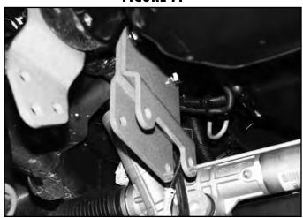
40. Install the driver's side rear differential drop bracket (01238) to the frame with three 12mm x 30mm bolts and ½" SAE washers (BP #617) into the existing welded nuts on the frame. (Fig. 12) The bracket will offset toward the outside of the vehicle with the gusset to the front. Leave hardware loose.
