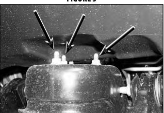
23. Loosen the strut-to-lower control arm hardware (Fig 4). Remove the nut from the bolt and leave the bolt in place to temporarily retain the strut to the lower control arm. Retain the nut.
