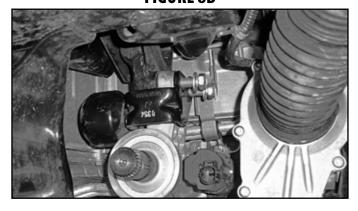
35. With the differential securely supported, remove the remaining bolts and lower the differential from the vehicle.
