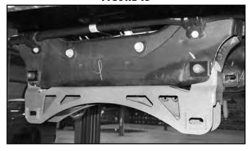
45. Install the new rear crossmember (01296) in the OE rear lower control arm pockets and loosely fasten with the provided 18mm x 150mm bolts, nuts in conjunction with the provided rectangle cam slot washers (01264). Run the bolts from front to rear and leave loose at this time. (Fig. 14)
