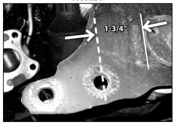
37. Install the provided passenger's side differential drop bracket (02389B) to the original frame mount with OE hardware. The brackets should be installed offset forward as shown (Fig 10). Leave hardware loose.
