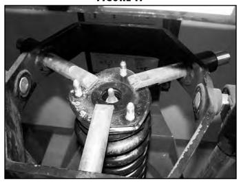
52. Place the provided preload spacer (01278) between the plastic coil seat and the rubber isolator (Fig 18).
