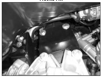
39. Install the driver's side rear differential drop bracket (01238) to the frame with three 1/2" x 1-1/2" bolts and ½" SAE washers (BP #660). (Fig. 12) The bracket will have the gusset plate towards the front of the vehicle. Leave hardware loose.
