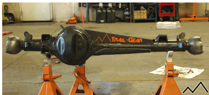
Front Gusset and Armor Installed
