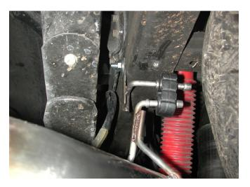
**Step 5.** Install the hanger bracket on the driver's side using the predrilled hole in the frame as shown.
