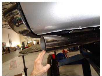
**Step 6.** Install the Tail Pipe Assembly in the same way. The Outlet may be trimmed as desired.
