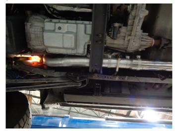
**Step 2.** Install the corresponding Inlet Pipe Assembly and loosely fasten it to the turbo charger outlet using the OEM clamp. Next, loosely attach the Inlet Pipe Lower Assembly to the Inlet Pipe Assembly using the supplied clamp. Refer to the table below to select the appropriate extension pipes for your vehicles configuration.
