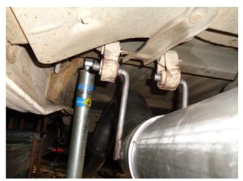
**Step 4.** Loosely install the Y-Collector and Over Axle Pipe Assemblies using the supplied clamps. Locate both welded hangers to the rubber insulators.
