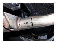
2. To remove stock exhaust, measure 2.5" from exhaust hanger located before the 2bolt flange. See picture. Remove stock exhaust from the 3 rubber hangers. Use WD-40 to aid in removal.
