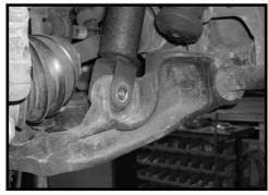
3. Working on the driver side, scribe a mark on the lower control arm and one directly across to the torsion bar. This will ensure that the torsion bar gets installed properly back into the OE location.
