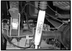
23. Locate the (2) 1/4" USS flat washers that are packaged with the installer copy of the installation manual. Working on the driver side rear shock bracket, re-install the stock bracket line bracket to the rear shock bracket using the OE hardware and the 1/4" USS washers as spacers. This will ensure that the shank of the bolt will not rub on the new shock.
