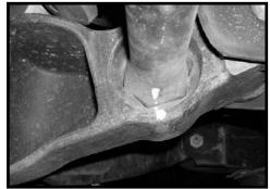
4. Working on the driver side and using a proper torsion bar removal tool. Carefully remove the torsion bar bolt and block. Set the torsion bar bolt and block aside. Remove the stock torsion bar unloading tool from the stock cross member. Special note: Tuff Country EZ-RIde Suspension requires that a proper torsion bar unloading tool be used when performing this installation. If you do not have one, please contact your local GM dealer to purchase one from them.
