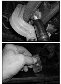
5. Working on the driver side, tap the torsion bar forward until the torsion bar key can be removed. Remove and discard the torsion bar key.
