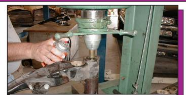
OWER CONTROL ARM BUSHING REMOVAL: There is no outer metal shell to press out. The rubber bushings are bonded to the inner sleeve, but not the control arm. Press the bushing/sleeve out as a unit. Use spray lube to help remove the old rubber bushings from the lower control arms.
