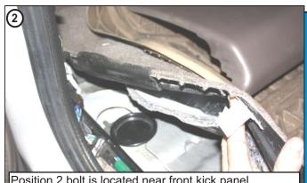
Position 2 bolt is located near front kick panel. Remove the plastic door trim and kick panel, pull up carpet and remove the black round plug.
