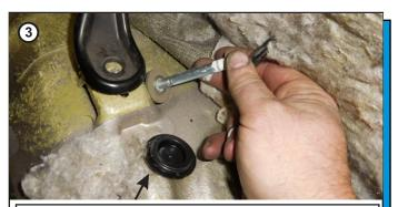
Position 3 bolt is located under the front seat next to the rear mounting point. Remove the 4 mounting bolts and lift the seat up and pull up carpet and remove the black round plug. Black round plug already removed.
