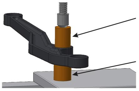
Inside diameter of control arm front 2 positions is 2.360" (60mm). Push out old metal shell with something smaller than 2.360". Inside Diameter of control arm rear position is 2.125" (54mm). Push out old old metal shell with something smaller than 2.125".
