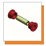
Note: Remove old bushings, clean ID of the control arm eyes. Apply a light coat of "Formula 5" grease to I.D, O.D. and Flange of the bushing. Apply a light coat of grease to the OD of the sleeve. Reassemble the bolt and torque to factory specs.
