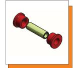
Note: Remove old bushings, clean ID of the control arm eyes. Apply a light coat of "Formula 5" grease to I.D, O.D. and Flange of the bushing. Apply a light coat of grease to the OD of the sleeve. Reassemble the bolt and torque to factory specs.
