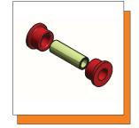
Note: Remove old bushings, clean ID of the control arm eyes. Apply a light coat of "Formula 5" grease to I.D, O.D. and Flange of the bushing. Apply a light coat of grease to the OD of the sleeve. Reassemble the bolt and torque to factory specs.
