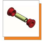
Note: Remove old bushings, clean ID of the control arm eyes. Apply a light coat of "Formula 5" grease to I.D, O.D. and Flange of the bushing. Apply a light coat of grease to the OD of the sleeve. Reassemble the bolt and torque to factory specs.
