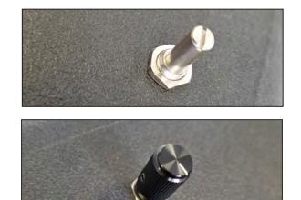
4. Find a suitable location to mount the sensitivity knob, drill a 3/8"id hole, remove the knob and install the rheostat then reinstall the knob.
