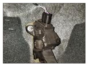
1. Locate the pedal wiring harness connection on top of the throttle pedal assembly and release the locking tab and disconnect the electrical connection.
