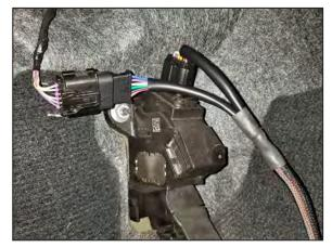
2. Connect the pedal module wiring harness into the pedal assembly and then connect the factory wiring harness into the pedal module wiring harness.
