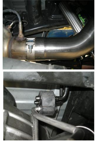
**Step 2.** Begin installation of the Magnaflow system by clamping the Inlet Pipe to the outlet of the DPF using a supplied 4.00" clamp and fitting the hangers in the rubber insulators (leave all clamps loose for final adjustment of the complete system).
