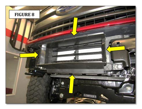
The air duct housing must be cut and a section removed from the bottom to allow clearance for the Winch Tray. Reference the measurements shown, (FIGURE 9). **Note:** Care must be taken not to damage the louvers when cutting the air duct housing.
