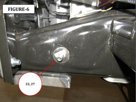
**Step-8** Secure the driver side support bracket to the frame using the bolt plate, (1) ½" flat washer, (1) ½" lock washer and (1) ½" hex nut. Attach the opposite end of the support bracket to the bumper shell bracket using (1) 3/8" x 1 1/4" hex bolt, (1) 3/8" lock washer, (2) 3/8" flat washers and (1) 3/8" hex nut, (FIGURE 7). Repeat steps 7 & 8 to install the passenger side support bracket.
