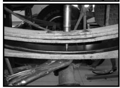
Working on the driver side and using a die grinder, carefully cut off the excess thread from the new centering bolt. new shocks, install the new bushings and proper sleeves Repeat procedure on the passenger side.
