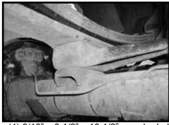
ers from hardware bag 916NW. Also, locate the stock upper u-bolt plate. Working on the driver side, secure the axle to the stock spring using the new u-bolts, u-bolt hardware and stock u-bolts plates. Torque to 110 ft lbs. Repeat procedure on the passenger side.
