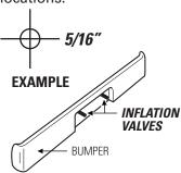
Install inflation valve assembly as shown.
