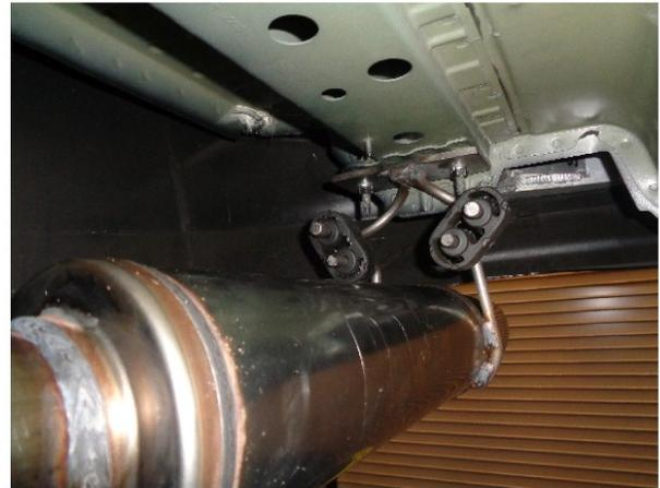
**Step 4:** Using the existing studs located on the factory frame rail mount the supplied Hanger Assembly with the supplied M8 lock nuts and washers.
