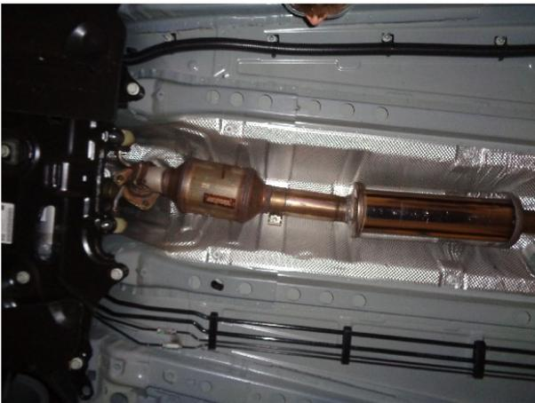
**Step 2:** Begin installing your new system by sliding the Resonator Assembly over the cut pipe and loosely attaching with the provided 2.38" clamp. Engage the hanger to the rubber insulator.
