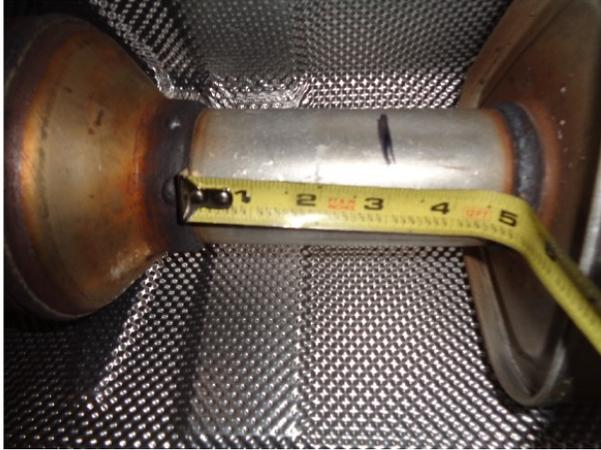
**Step 1:** To install the MagnaFlow exhaust the OE system must be cut. Measure 3.00" back from the catalytic converter weld, cut at this point and deburr pipe. Working front to rear disengage all welded hangers from the rubber insulators. The OEM exhaust system can now be removed in one piece. Be sure to retain the rubber hanger insulators as they will be needed to install your new MagnaFlow system.
