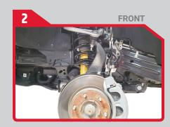
· Tie rod end, sway bar link end, upper ball joint, and the cv axle nut need to be unbolted to properly remove and install front coilover assemblies.
