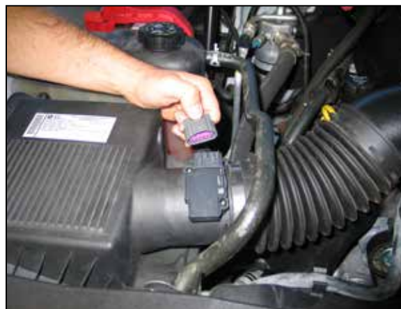
2. Disconnect the mass air sensor electrical connection.
