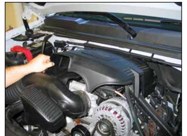
3. Lift up and remove the engine cover from the engine as shown.
