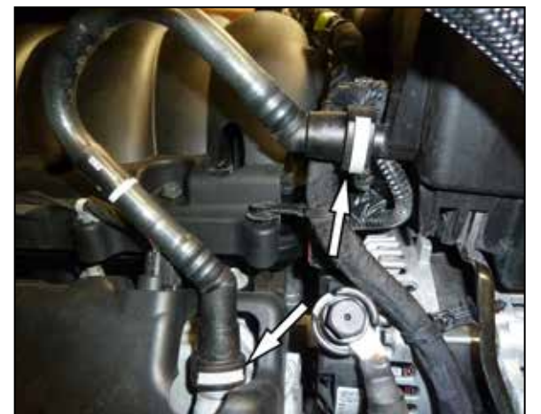
3. Depress the locking tabs and then disconnect the crank case vent line from the intake plenum and valve cover vent port.
