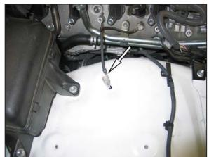
8. Remove the bolt that secures the ground strap to the inner fender.
