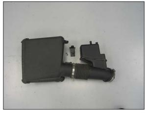
17. Remove the two screws securing the mass air sensor and then remove the mass air sensor from the upper air box housing.
