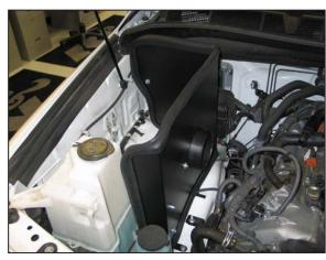
14. Set the heat shield into the engine compartment and secure the factory install nuts with the provided hardware. **NOTE:** Be sure to place the ground strap between the mounting bracket and the inner fender and then secure with the heat shield mounting bolt.
