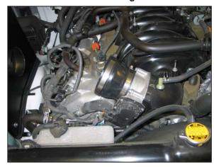
15. Install the silicone hose (08050) onto the throttle body and secure with the provided hose clamp.
