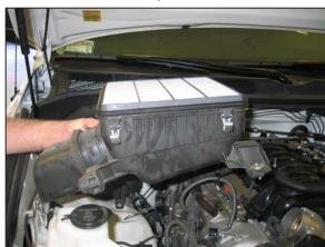
7. Loosen the two bolts securing the lower air box and then remove the lower air box from the vehicle.
