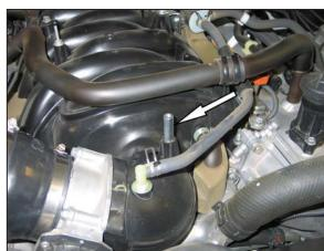
30. Install the provided nut extension onto the stud as shown.
