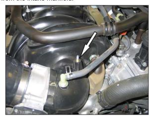
29. Install the provided stud into the mounting stud location as shown.
