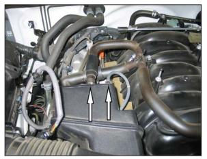
5. Disconnect the crank case vent hose and fuel pressure line from the intake resonator.
