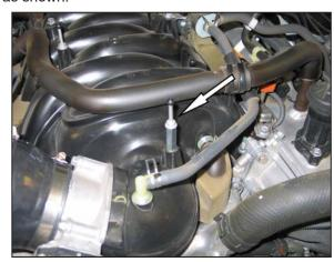
31. Install the mounting stud into the nut extension as shown.
