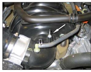
28. Remove the front engine cover mounting stud from the intake manifold.
