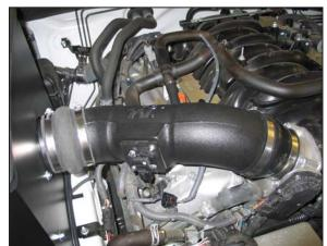
24. Install the K&N intake tube into the hump hose at the heat shield and then into the step hose at the throttle body and secure with the provided hose clamp.
