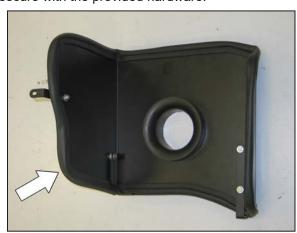
13. Install the provided edge trim onto the heat shield as shown. **NOTE: Some trimming of the edge trim will be necessary.**
