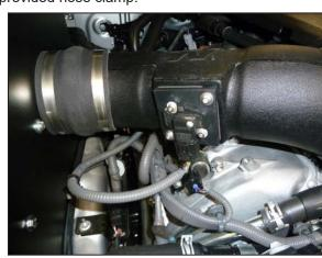
27. Reconnect the mass air sensor electrical connection.
