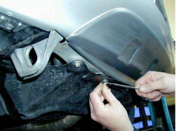
• Remove the 4 bolts retaining the lower bumper bar.
