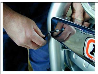
Remove plastic film from driving light panel, fit ARB domed badge and assemble to the nudge bar using 4 M6 button head bolts and flange nuts supplied. You will need a 4mm allen key for this step.
