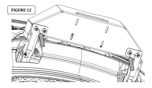
**Step-11** Hold one of the grille guard side plates up in position on the outside of the upper and lower mounting brackets. Fig 13.
