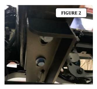
**Step-3** Place the main bracket were you removed the tow hook. Re-attach using the factory bolts removed in previous step. Figure 2. Leave loose. Follow to step 7.
