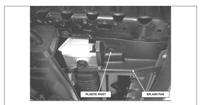
STEP 1. REMOVE THE RIVETS, AND PLASTIC SPLASH PAN FROM THE BOTTOM OF THE VEHICLE.
