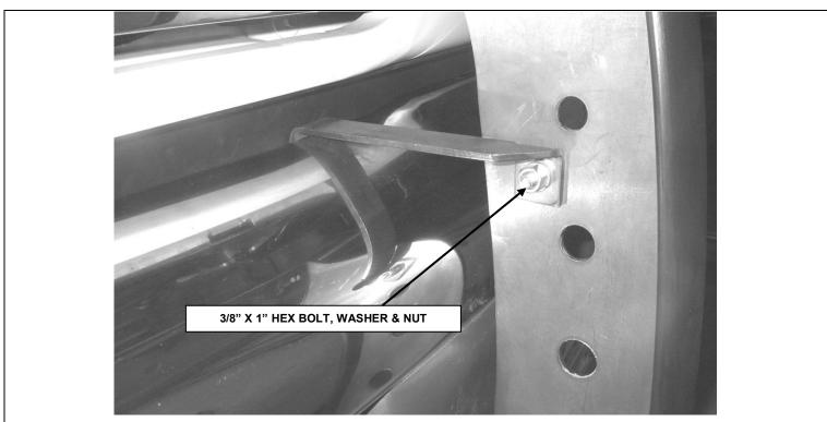
**STEP 7.** ATTACH THE GRILLE GUARD ASSEMBLY TO THE UPPER BRACKETS USING THE 3/8 X 1" HEX BOLTS, WASHERS AND NUTS.
