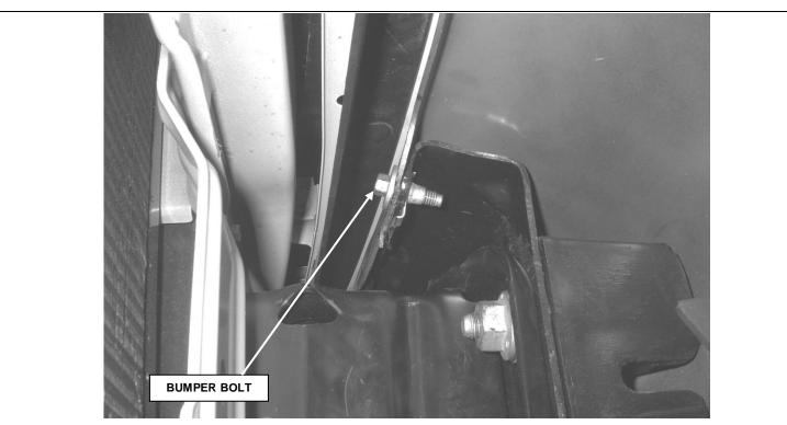
**STEP 2.** BEGINNING WITH THE **DRIVER SIDE**, REMOVE THE UPPER BUMPER BOLT. THE BOLT IS LOCATED ON THE BACK EDGE AT THE TOP OF THE BUMPER. THIS LOCATION WILL SERVE AS THE UPPER BRACKET MOUNTING POINT.
