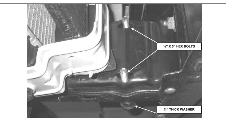
**STEP 4.** LOCATE THE TRIANGULAR SHAPED HOLES IN THE FRAME RAIL. USING THE ½" X 5" HEX BOLTS AND ½" THICK WASHERS SLIDE THE BOLTS THROUGH THE FRAME SO THE THREADS ARE FACING TO THE CENTER OF THE VEHICLE.
