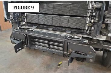
**Step-14** With both brackets installed, leave a center distance of 27 ¾"-28" in between. Brackets should be finger tight to allow for adjustment when installing the center bumper section. Figure 10.
