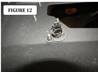
**Step-17** Remove the parking sensor bezels from the OEM bumper by depressing the tabs around the base and pushing the bezel out through the front of the bumper.
