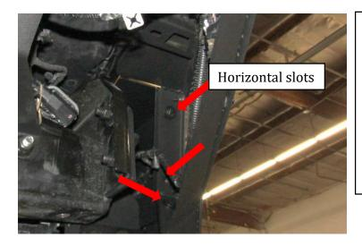
**Step-25** Adjust your bumper to square up with the front end and fasten any loose hardware accordingly. The bumper should not make any contact with the OEM bumper or grill. It should have an approximate ½"-½" spaced away from the OEM bumper The wings of the bumper should line up where the fender and OEM bumper meet. If you should find that the Element bumper is making contact, evaluate where it and adjust the bumper as needed.
