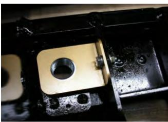
24. When the large nut is in its final position, secure with the nut retaining bracket using an M6 bolt, washer and flange nut.
