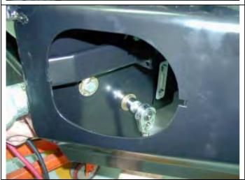
41. When bar is aligned, tighten bolts.
