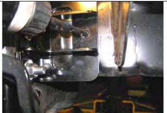
9. Drill 1 x M10 pinning hole in chassis using existing hole in reinforcing bracket as a guide.
