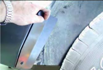
56. Fit liner retainer bracket with black M6 bolt and washer sets into M6 cage nuts in wing returns each side as shown.
