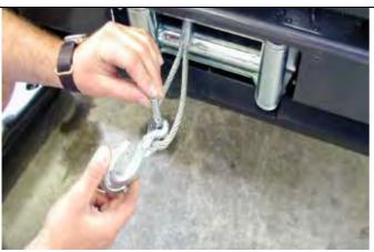
54. If winch fitted, fit off winch hook.
