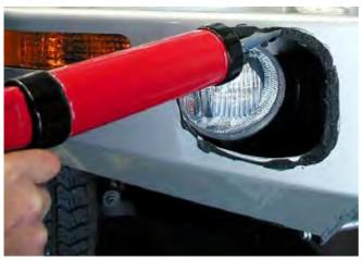
51. Note that the aperture moldings are handed (RH or LH), select correct hand for each wing aperture. Apply Sikaflex to recess in aperture molding flange then fit to aperture in wing. Use adhesive tape to secure plastic mold while Sikaflex cures.
