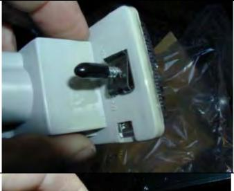
19. Remove lights from cartons and then remove screws and speed nuts from each light. These fasteners are not to be reused – new screws are supplied in the fitting kit
