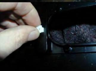
20. Insert nylon nuts into square holes in light brackets inside wing area
