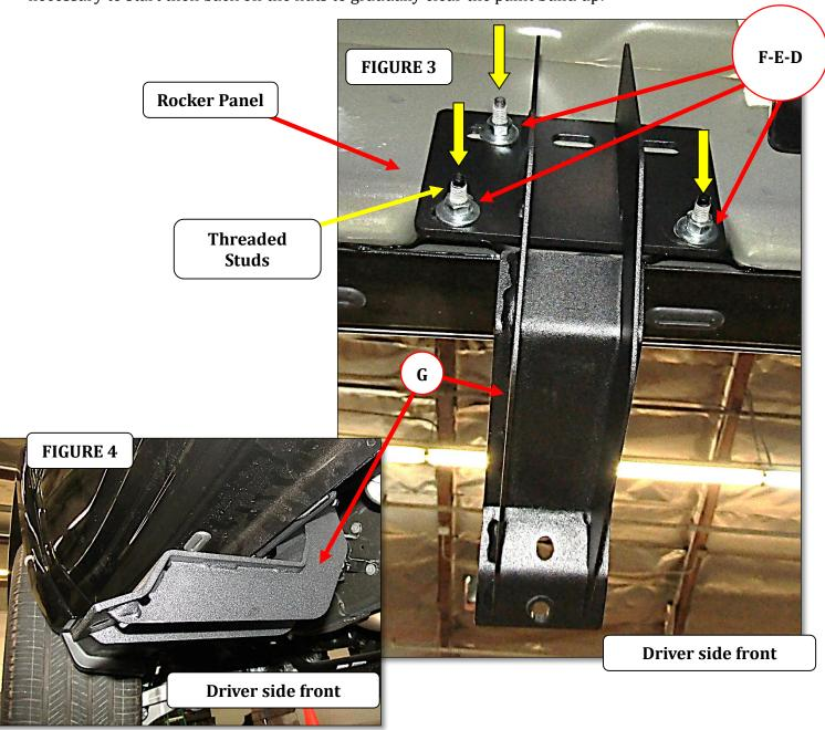
**Step-3** Locate the (3) threaded studs on the inner rocker panel at the center and rear of the cab and repeat step 2 to install two of the brackets using the supplied hardware. Note: The front mounting location is shown in Figure 3. The center and rear mounting locations are similar.
