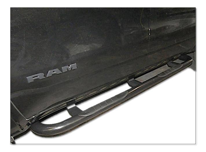
**Step-6** Repeat the installation steps to install the mounting brackets and step on the driver side. Remember to check and retighten all nuts and bolts periodically.
