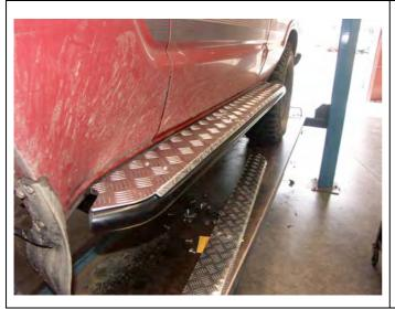
7. Place the aluminium step plates on the side steps and fix in place using the M6 x 25mm coach bolts, M6 panel washers and M6 flange nuts.
