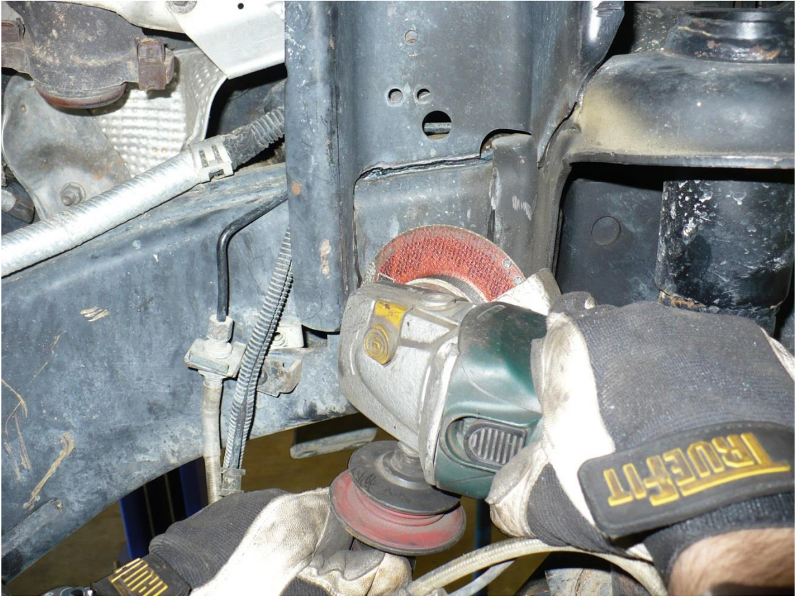
b) Cut the front of the shock mount where it attaches to the coil mount
