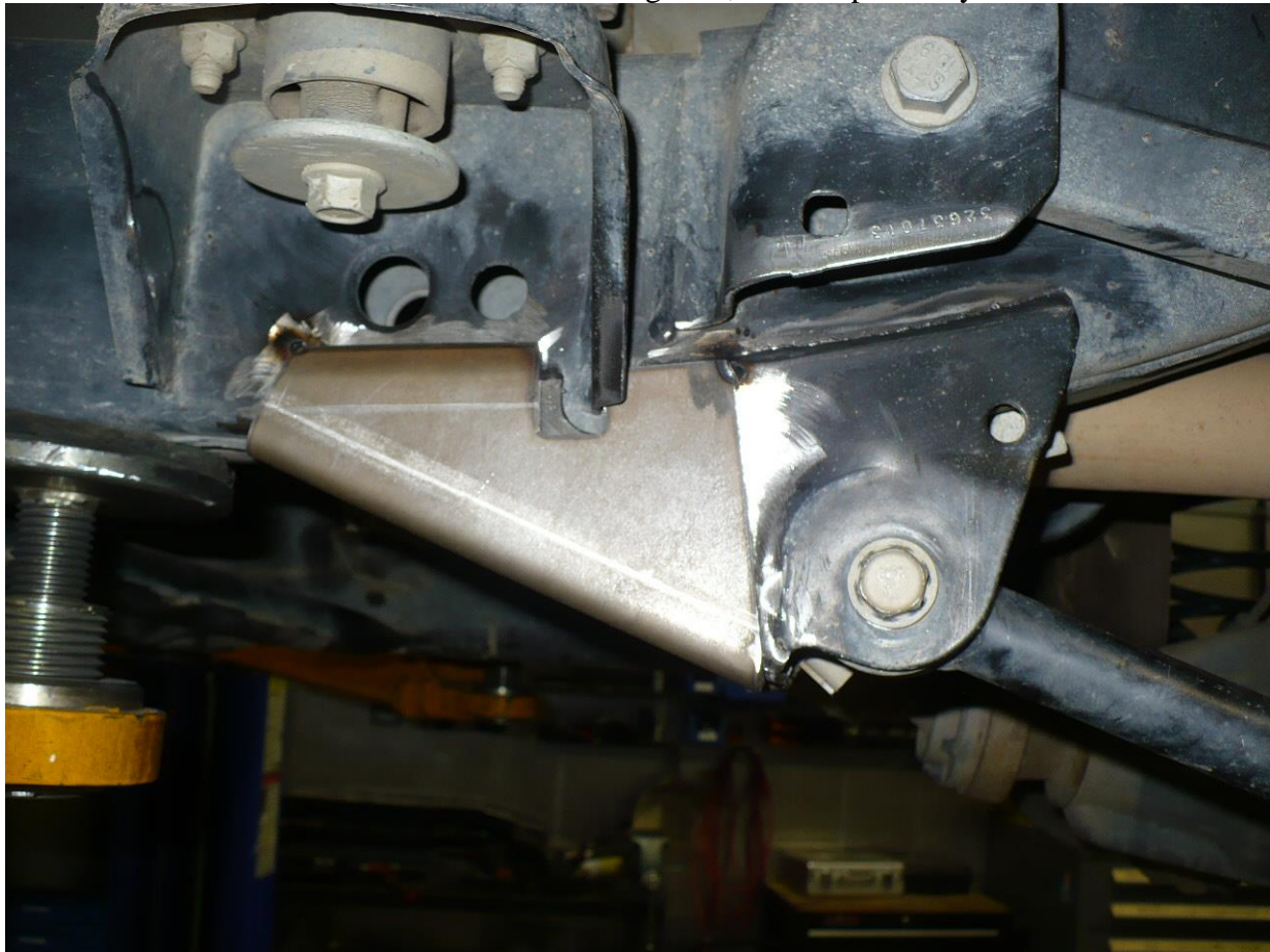
IMG. 2.2 Placement of 502202-01 RLCA outer gusset
