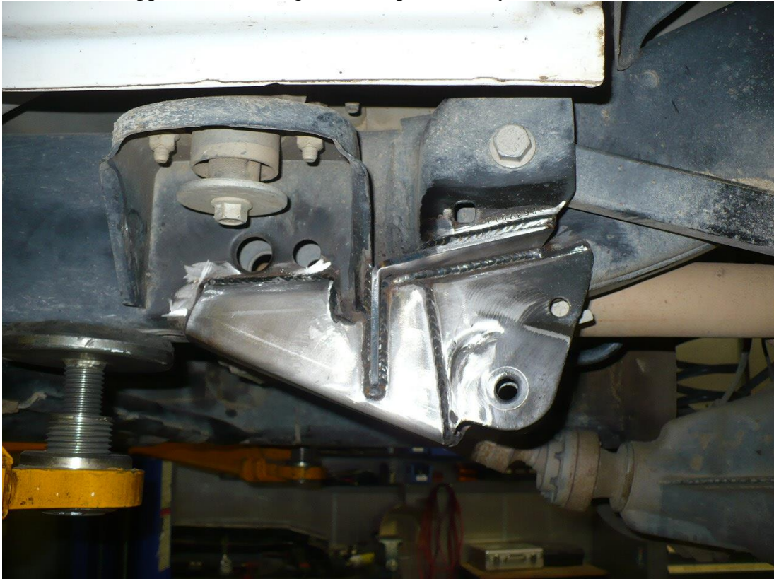
5) Tack 502202-02 rear upper control arm gusset into place. Fully weld once desired fitment is achieved.
