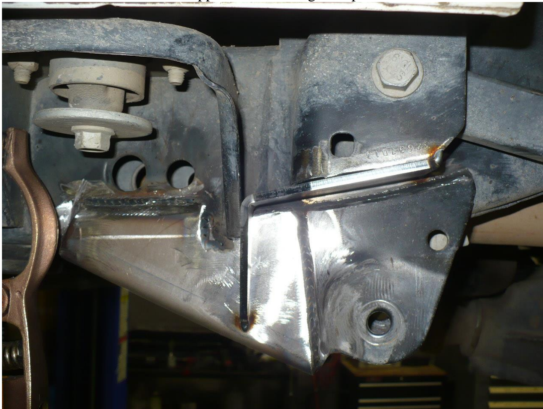
IMG 3.2 Reference for Upper control arm gusset placement.
