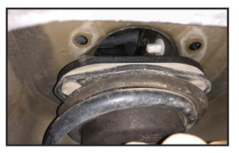
4. Once the new spacers have been installed, carefully raise both sides of the front suspension so that the upper strut studs go back through the original holes of the vehicle.
