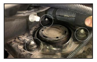
3. Locate the new strut spacer plates and install 1 each on top of the OE struts over the 3 studs. **Special Note: the Spacer will only go on one way, so if at first it does not line up with the studs, re-orient the spacer until it does.**
