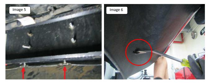
5. Locate and remove the factory bolt shown. Place auxiliary mounting bracket and secure usgin the bolt removed. Do not tighten. Image 7 y 8.
