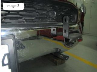
3. Place (2) 1/2" tab bolts from front of the main bracket to rear. Secure the main bracket to the bumper support using (2) 1/2 hex nuts, (2) ½" flat washers and (2) ½" lock washers. Image 3 & 4. **Note:** Leave the nuts loose for final adjustment.
