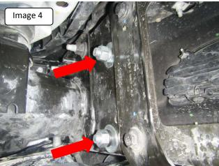
4. Remove the air dam by removing the bolts and push pin rivets. Image 5 y 6.
