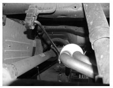
ATTACH HANGER #E INTO RUBBER GROMMET LOCATED JUST ABOVE DRIVERSDE TAILPIPE ASSEMBLY, SLIDE THIS CLAMP OVER DRIVERSIDE TAILPIPE. DO NOT TIGHTEN.
