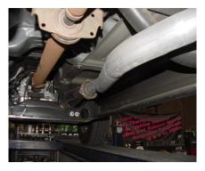
TO REMOVE STOCK EXHAUST UN-BOLT IT FROM THE 2-BOLT FLANGE LOCATED JUST BEHIND THE Y-PIPE. **DO NOT DAMAGE THE FACTORY HARDWARE, YOU WILL RE-USE IT.** NOW CUT OFF YOUR STOCK TAILPIPE JUST BEHIND THE MUFFLER AND REMOVE. LEAVE ALL RUBBER GROMMETS ON THE HANGER. USE WD-40 TO AID IN REMOVAL OF EXHAUST AND HANGERS.
