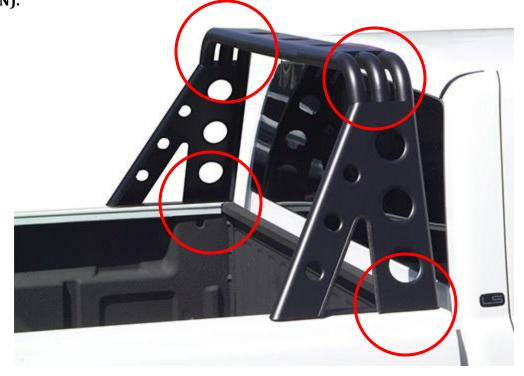
(Optional Attachment) Drill the bed rails and attach the sport bar using the 3/8" bolts washers and nuts supplied.
