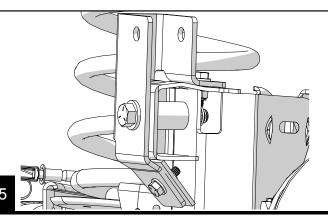
Lower the vehicle to the ground. Place the track bar into the new bracket, and install the factory nut and bolt. Torque to 75 ft-lbs.
