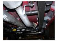
3. Install headpipe #A onto your existing stock front headpipe using stock hardware to secure pipes together. Do not tighten. Insert welded hangers into rubber grommets.
