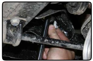
7. Remove sway bar links using an 18mm socket and wrench, make sure to put aside for use in the front of the vehicle.
