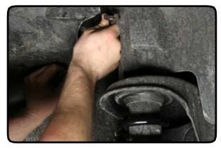
24. Remove sway bar links using 18mm socket and wrench at the axle and 18mm socket and 20mm wrench at the sway bar. Lower the jack enough to remove the springs.
