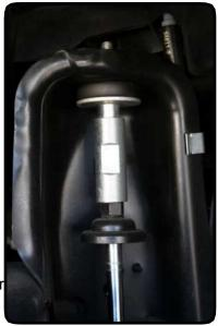
Install factory rear sway bar links in the front on the outside of the sway bar and inside of the axle mount. Torque to 75 ft-lbs.
