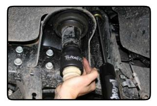
30. Install the factory coil springs. Do the drivers side first.
