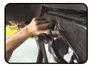
17. Install new rear bump stop spacer by placing the spacer on the axle pad lining up both holes with the overhang part of the pad facing forward. Use the provided  $5/16^{\circ} \times 1 \frac{1}{4}^{\circ}$  bolts with  $5/16^{\circ}$  washers and  $5/16^{\circ}$  nuts. Tighten with  $1/2^{\circ}$  wrenches.
