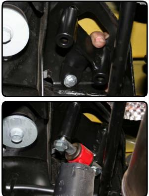
19. Install rear brake line extensions provided in the kit. Bolt the bracket to the factory brake line bracket by removing the 10mm bolt and installing the bracket in that location with the bend of the bracket going flush with the frame. NOT STICKING OUT AWAY FROM THE FRAME. Torque to 14 ft-lbs. (If bracket gets installed the wrong way it will rub on your tires) Then use the supplied hardware to attach the factory bracket to the drop bracket by using 1/2" socket and wrench.
