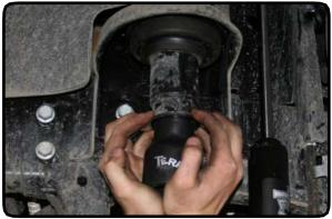
29. Use grease to lube the yellow bump stop and install it into the extension.
