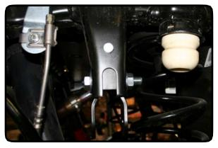
14. Install the factory isolator onto the new TeraFlex rear spacer. Install the new spacer into the frame. You should feel or hear a popping and the spacer should stay hanging from the frame.
