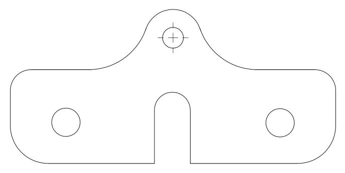
Cut this template out and bolt it on the outside of the factory track bar bracket. Use tape to ensure that the template does not move and center punch the top hole for the new TeraFlex track bar drop bracket.
